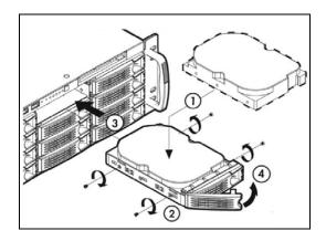
① Press the blue button, hold the pull rod to pull out the HDD case and then install the HDD into the case.
